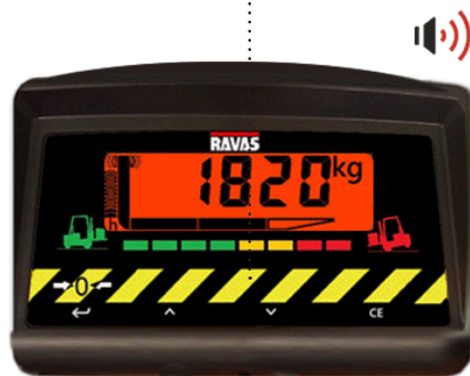
Overload situation: tip loading
