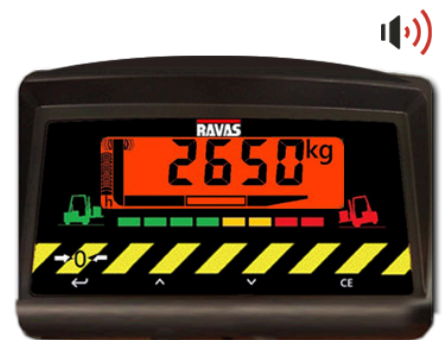
Overload situation: load too heavy
