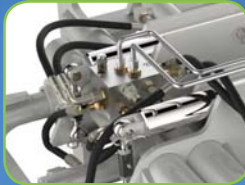
Cross over relief to prevent over clamping
